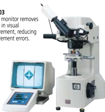
HM-113 Reduce individual differences in visual measurement with the TV monitor. The statistical calculation function reduces operation time.
