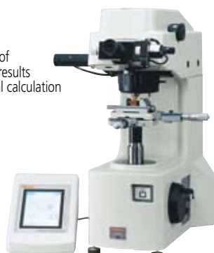
HM-113 Reduce individual differences in visual measurement with the TV monitor. The statistical calculation function reduces operation time.
