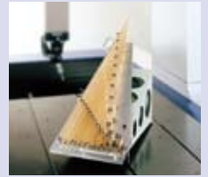
CMM calibration using a virtually zero thermal expansion glass gage
